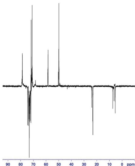
Figure 1 ^{13}\text{C} -DEPT spectrum of polymers of GPTS obtained from polymerization with KOH at 40^\circ\text{C} . [Color figure can be viewed in the online issue, which is available at wileyonlinelibrary.com .]
